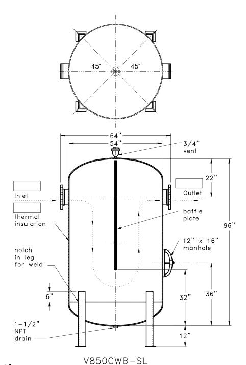
(4) 4"x4"x1/2" steel angle legs and 6"x6"x1/2" baseplates w/ 3/4"ø hole in each plate on 62-5/8" boltcircle
