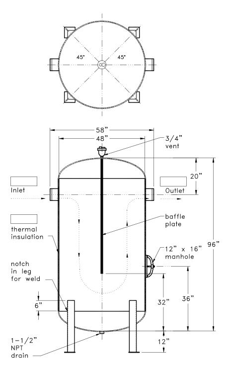
(4) 4"x4"x1/2" steel angle legs and 6"x6"x1/4" baseplates w/ 3/4"ø hole in each plate on 56" boltcircle
