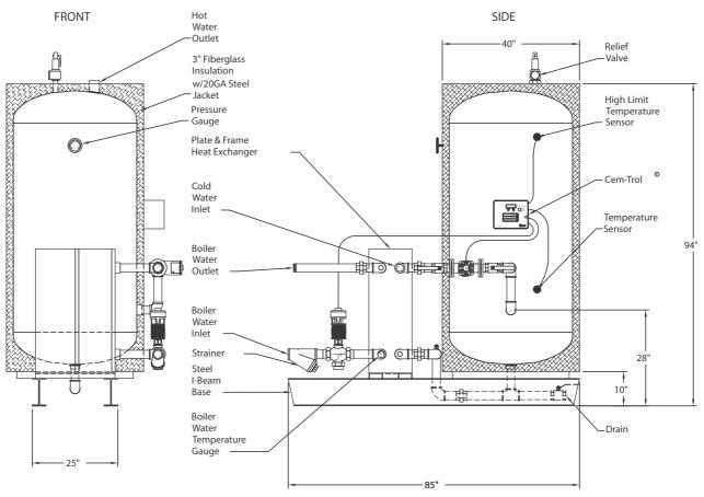
V300SPH-PF-2W PLATE & FRAME HEAT EXCHANGER
