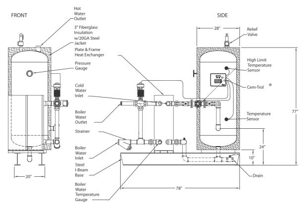
V120SPH-PF-3W PLATE & FRAME HEAT EXCHANGER
