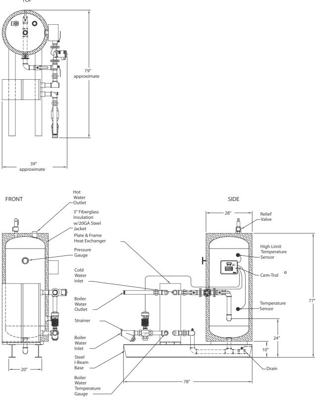
V120SPH-PF-2W PLATE & FRAME HEAT EXCHANGER
