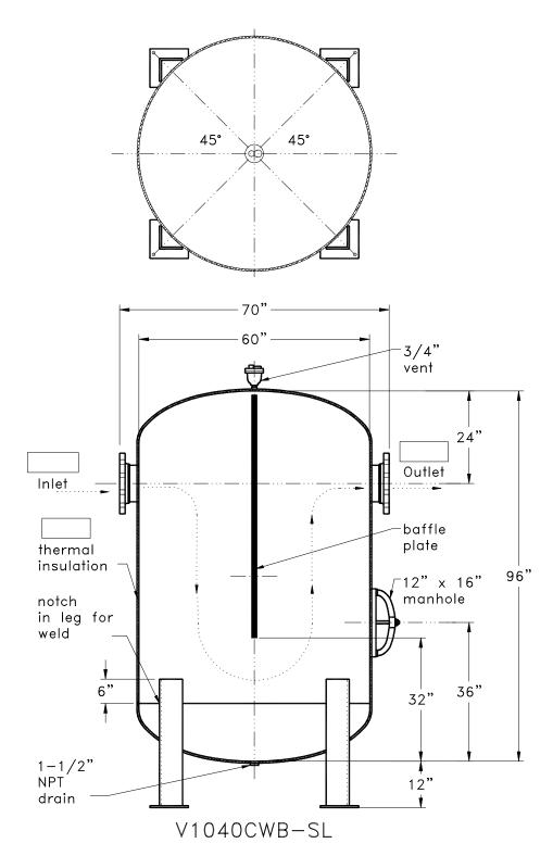
(4) 6"x6"x1/2" steel angle legs and 10"x10"x1/2" baseplates w/ 3/4"ø hole in each plate on 74" boltcircle
