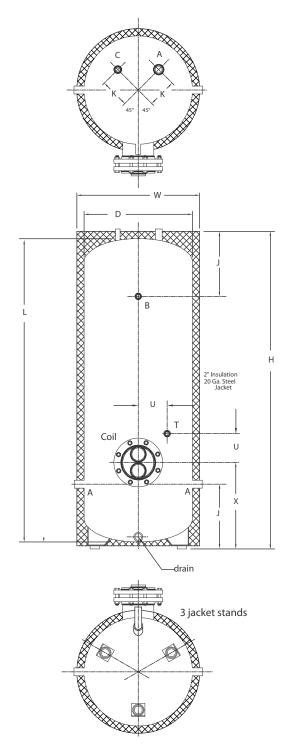
3 Legs - Less than 42" dia. and/or 96" height 4 Legs - Greater than 42" dia and/or greater than 96" in height
