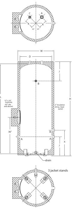
3 Legs - Less than 42" dia. and/or 96" height 4 Legs - Greater than 42" dia. and/or greater than 96" in height
