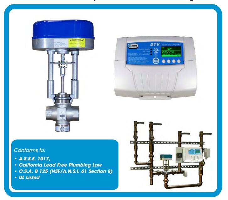
The Cemline® Digital Tempering Valve (DTV) is designed to provide consistent tempered water to institutional and commercial facilities. The digital controller wired to the stainless-steel control valve can accurately maintain set point within +/-2°F from 0.5 gpm to full flow. The DTV series can be used for domestic hot water, or heating/cooling for industrial applications. The controller can
