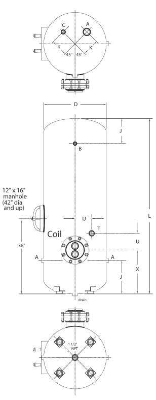
24" dia to 36" dia - 3 leg clips 42" dia to 96" dia - 4 leg clips
