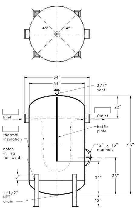
(4) 4"x4"x1/2" steel angle legs and 6"x6"x1/2" baseplates w/ 3/4"ø hole in each plate on 62-5/8" boltcircle
