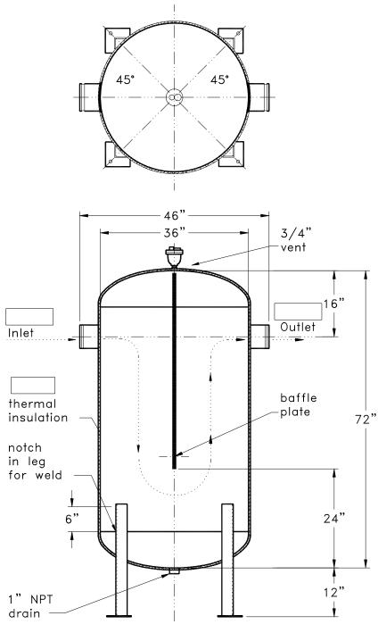
(4) 3"x3"x1/4" steel angle legs and 6"x6"x1/4" baseplates w/3/4"ø hole in each plate on 44" boltcircle
