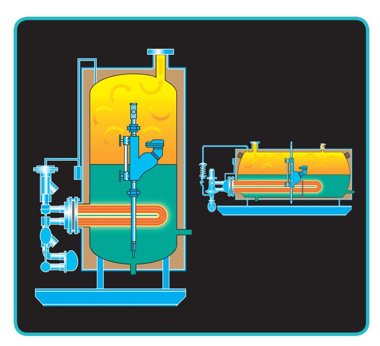
Cemline Unfired Steam Generators are designed to produce clean steam with steam or high temperature hot water as an energy source for use where there is a need to produce clean steam.
