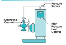
**(Energy Source-Steam):** A pilot operated steam control valve uses a steam pilot to monitor output steam pressure and automatically modulate the flow of source steam to maintain a constant output steam pressure. A pilot operated controller is field adjustable.
