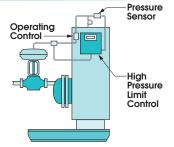
**(Energy Source-HTHW or Steam):** A pneumatically (air) operated steam control valve uses building air connected to a furnished transmitter which monitors the output steam pressure and sends a varying air signal to the source steam controller to modulate the flow of source steam to maintain a constant output steam pressure. Pneumatic set point is field adjustable.
